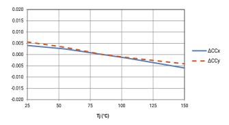
The following graphs represent typical chromaticity vs. current and temperature for the XLamp CXA2011 LED at 5000 K CCT.
