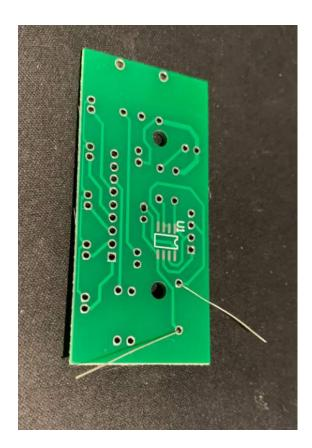
under the PCB, to avoid it moving around, to have an easier soldering environment
