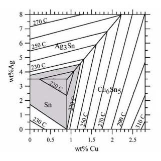
Eutectic point: Sn-0.3Ag-0.7Cu, melting point: 227°C
