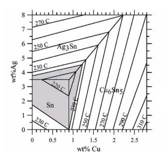
Eutectic point: Sn-3Ag-0.5Cu, melting point: 219°C
